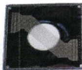
MMD: 64 strips, 100 μm pitch, 40 μm width, 1 μm thick
