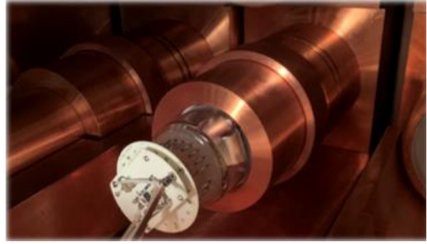
Fig. 2. Photo of the low-background voltage divider and pre-amplifier system mounted on the same board in DAMA/LIBRA-phase2-empowered. (See color Figure on the journal website.)
