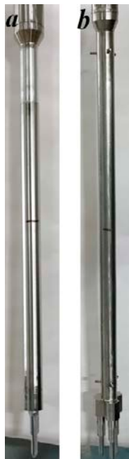
Fig. 2. Photographs of the material science vertical irradiation channels for irradiating surveillance specimens in the WWR-M reactor core: a - the smaller-diameter channel designed for a single fuel assembly; b - the larger-diameter channel designed for a triple fuel assembly.
