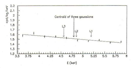
Cumulative experimental energy distribution (already corrected for the needed efficiencies) in the region of interest for the process searched for; the statistics is 19511 kg·day. The dotted line represents the result of a fit given by the sum of a linear function (simplified background model suitable for the present purposes) and of the sum of the three gaussians associated to the process searched for; this last contribution requires only one free parameter (see text).
